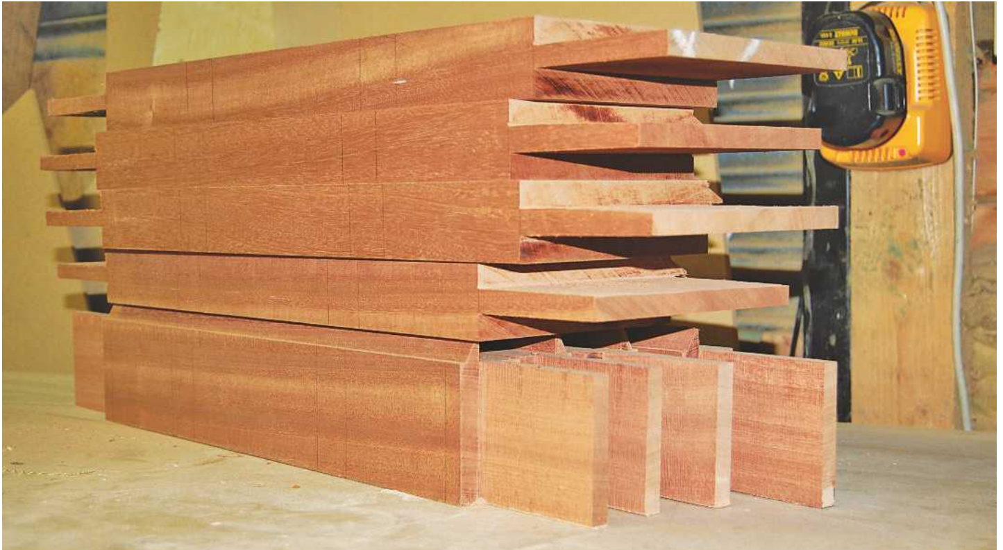
▲ Pic.10 A stack of tenons ready for haunching
